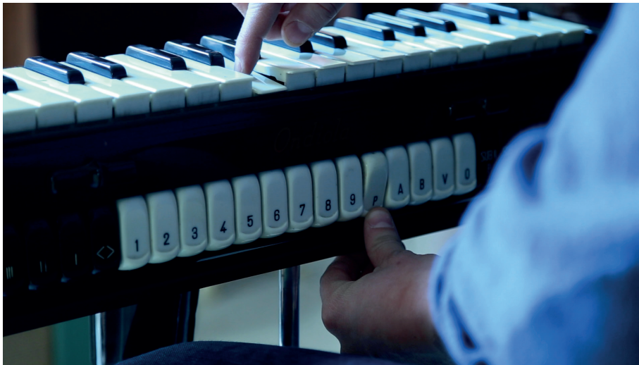
FIGURE 11. Sampling of Ondiola octave transposer, registers and volume controls. Author's personal video, recorded with permission of the Fondazione Isabella Scelsi. See https://youtu.be/f4xl8weTdTo
