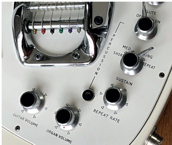
FIGURE 8. Detail of the Vox V251, showing the percussion knobs for the repeat function.
